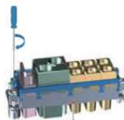
装配好模块后，闭合滑动边框，锁上螺丝 After finished assembly, close sliding border, lock screw
